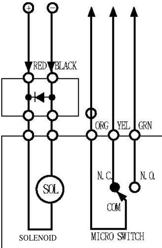
Because the voltage drop will result in being unable to drive the solenoid coil. Therefore, please make sure the thickness of the wire and the distance of the wiring, the voltage supply is good enough for normal operation.
